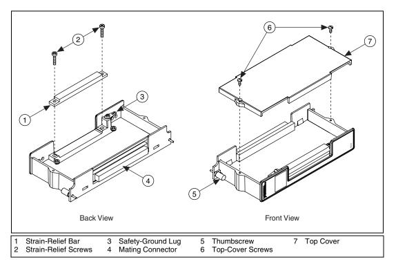
Figure 1. SCXI-1321 Parts Locator Diagram
